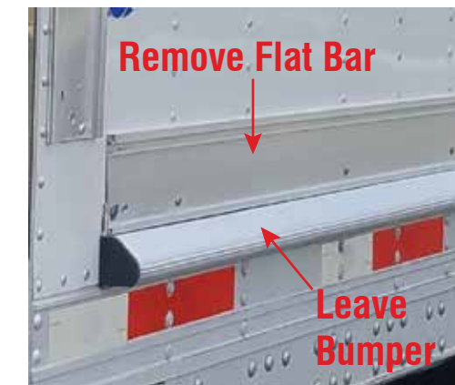
④ Detail of Existing Flat Bars TO BE REMOVED Scale: NTS
